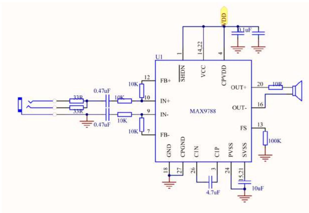
The above several schemes have a low voltage signal of 2.7~5.5V. If a higher power supply voltage signal is used, other schemes can be adopted.
